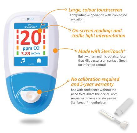
With just one touch of a button, a user can perform a test following the on-screen prompts for when to inhale, exhale and when to stop. The device analyses the amount of carboxyhaemoglobin (%COHb) and carbon monoxide levels (ppm) present in a breath sample with results displayed in seconds. PPM and %COHb values are shown as well as the familiar green, amber and red traffic light system providing the user with a visual interpretation of results.
