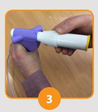
Insert the Spirette 'M' into the flow head. Attach adaptor and insert a clean one way valve mouthpiece.
