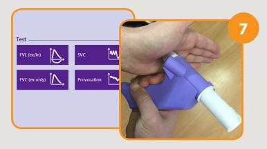
You have a choice of 5 tests. The only tests that you will use are "SVC" and "FVC" (ex only). To perform a slow VC first click on "SVC". On the next screen the ambient temperature etc will be shown. Click Confirm.
